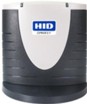
The 3121 USB landing desktop reader from Omnikey offers popular technology in a classic housing. This reader has landing contacts and is fully PC/SC and EMV Level 1 compliant and supports all ISO 7816 microprocessor-based smartcards as well as a variety of popular memory cards. It also meets USB 2.0 and CCID specifications for simple installation.
